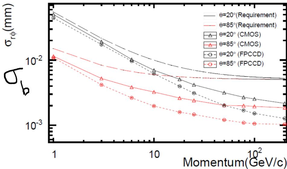
CMOS and FPCCD solutions meet the design requirement of  $\sigma_b = 5 \oplus 10 / (p \beta \sin^{3/2} \theta) \mu\text{m}$
