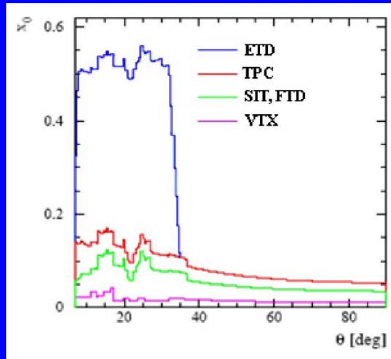
Forward tracking disks should ensure good quality track reconstruction to the edge of the TPC acceptance.
