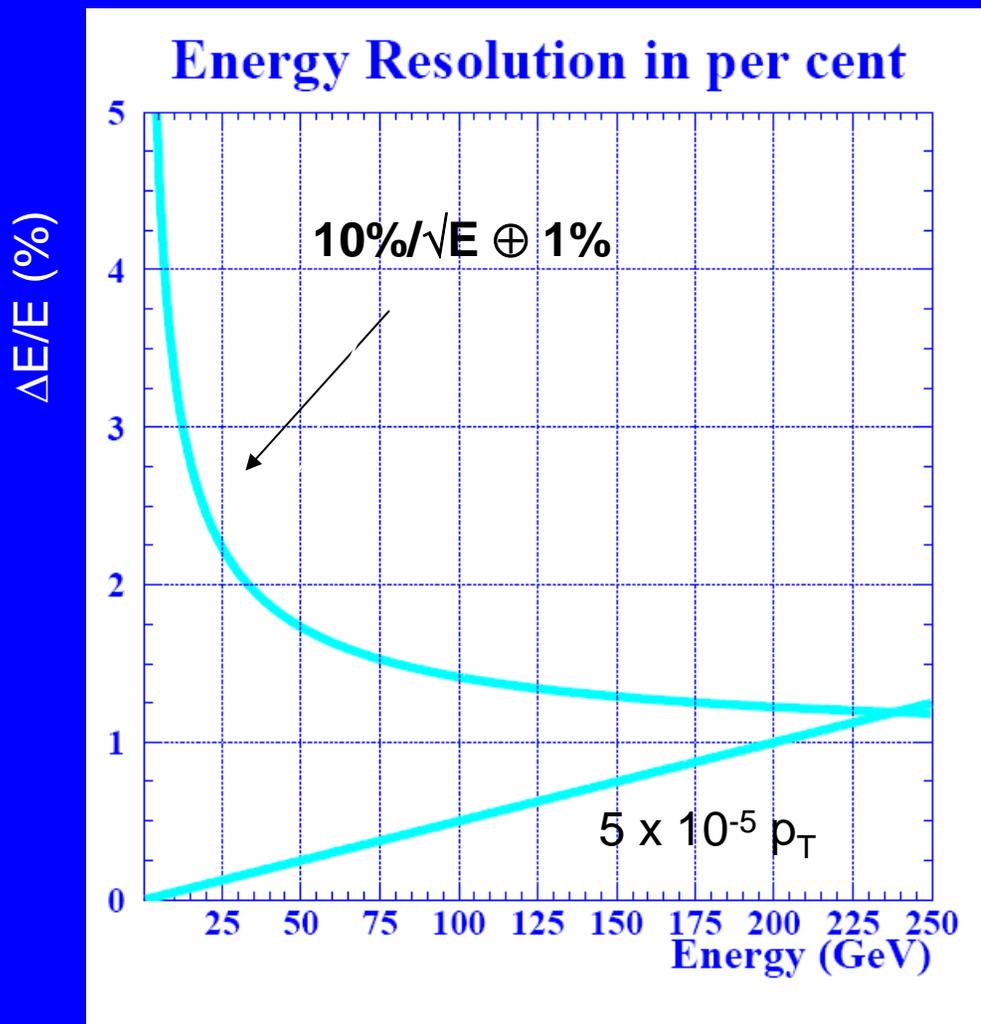
Even for electrons, the tracker should do better than the calorimetry ..... (modulo bremsstrahlung ....)
